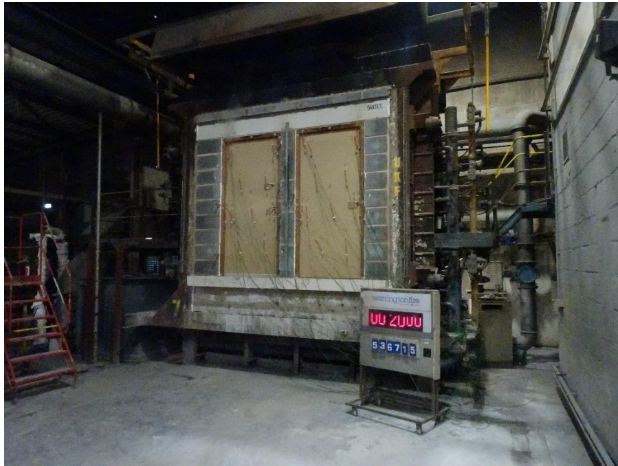
Figure 35 Unexposed face of the specimen at 20 minutes of testing
