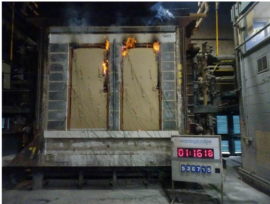
Figure 39 Unexposed face of the specimen at 76 minutes of testing
