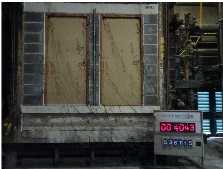
Figure 36 Unexposed face of the specimen at 40 minutes of testing
