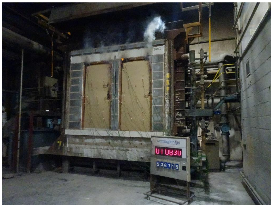
Figure 38 Unexposed face of the specimen at 68 minutes of testing
