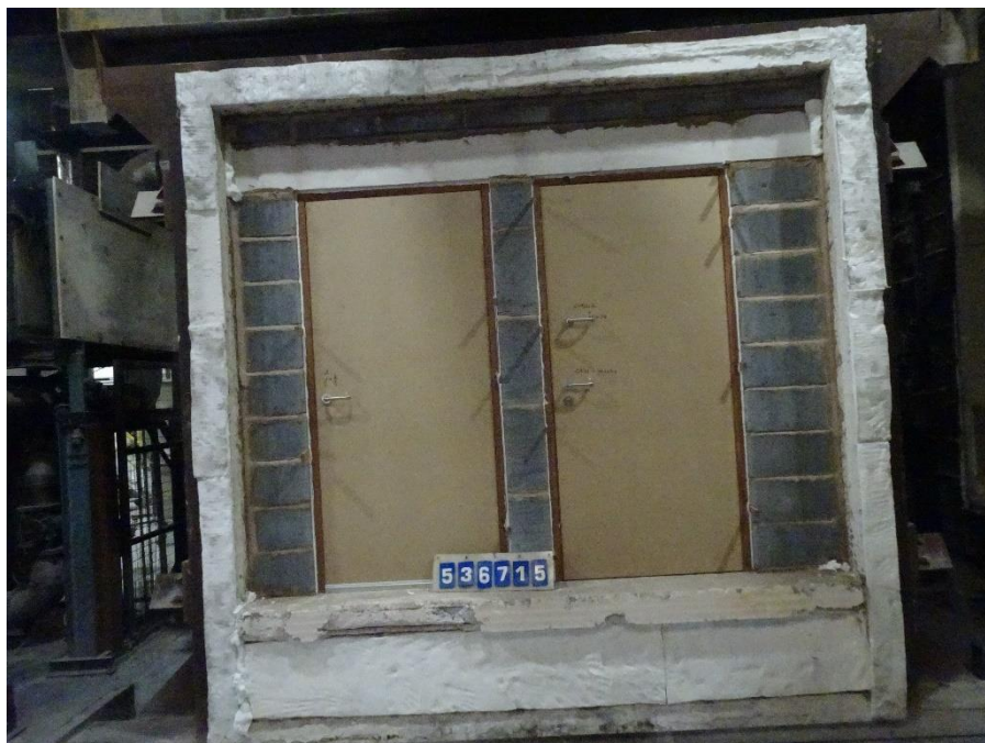
Figure 34 Exposed face of the specimen before the start of the test
