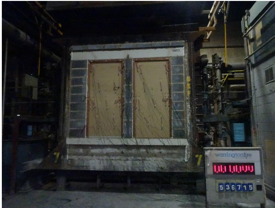
Figure 33 Unexposed face of the specimen before the start of the test
