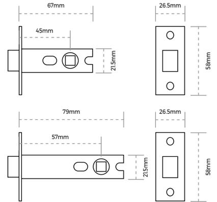
SPÅRKA fire rated tubular latches are designed for use with door handles and door knobs. Ideal for commercial and domestic use.
