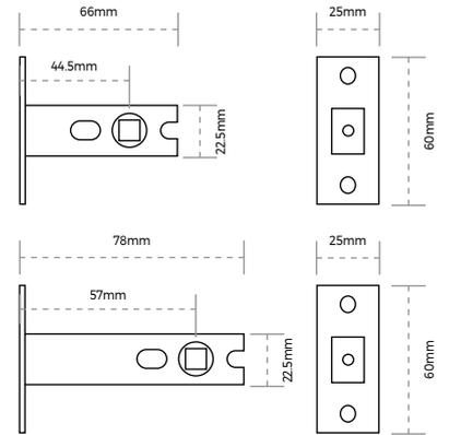
SPÄRKA heavy duty fire rated Tubular deadbolt are designed for use with bathroom thumb turns or lever on backplate with integrated thumb turn.
