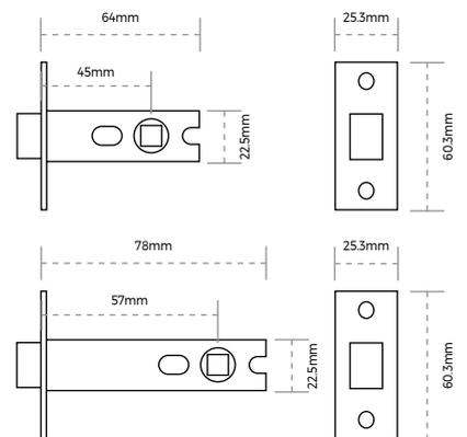
SPÅRKA heavy duty fire rated Tubular Latch are designed for use with door handles and door knobs.
