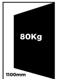
Rutland TS.5204 (S-20) Overhead Door Closer with cover is an EN variable power size 2-4 door closer making it suitable for doors up to 1100mm wide / or maximum 80 Kg. This door closer comes complete with mechanism, cover, armset, parallel arm bracket for mounting on the 'Push' face of the door, installation template and all fixings.
