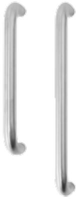
SPÄRKA 19mm Diameter Pull Handle, Supplied with bolt through fixings and is available with 225mm or 300mm centres.
