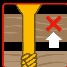
Partially Threaded Stops The Timber Jacking
