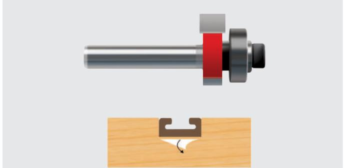
TCT Cutter 1/2" Shank for Centre Leg Pile Carrier
