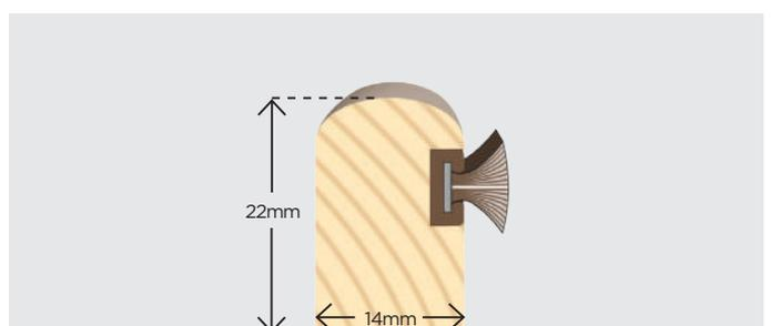
Timber Staff Bead 20mm x 15mm with Pile Carrier
