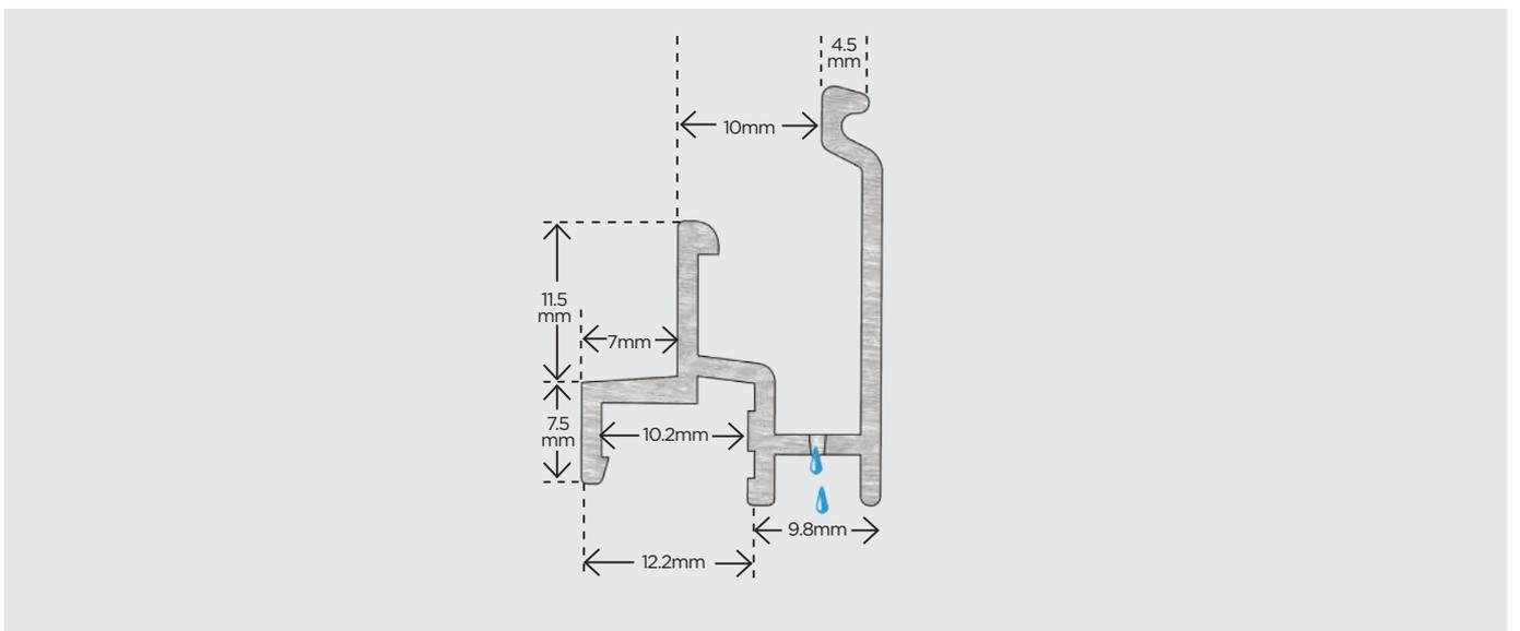
Glazing without external fixings, no damage to paint coating
