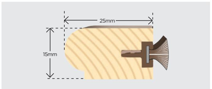
Timber Staff Bead 28mm x 15mm with Pile Carrier
