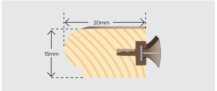
Timber Staff Bead 25mm x 15mm with Pile Carrier
