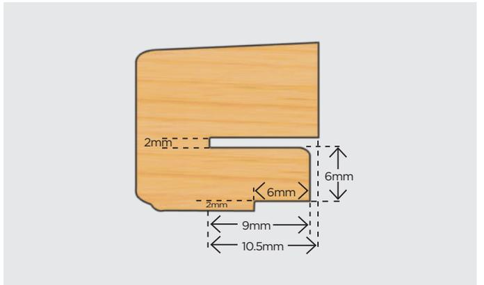
Automatically spaces the double glazed unit with a choice of 1mm to 6mm colour coded packer
