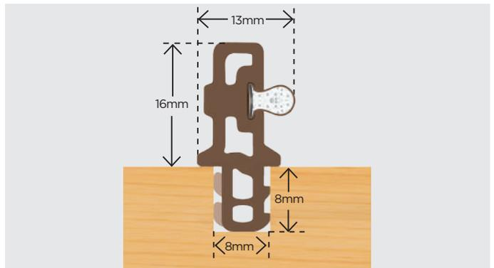
**Retaining Profile 10mm for Partex/Parflip**
