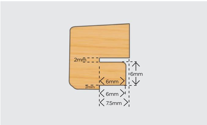
Securbead 9mm Anchoring Groove
