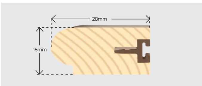
Timber Staff Bead 28mm x 15mm with Carrier & 6.5mm Pile & Fin
