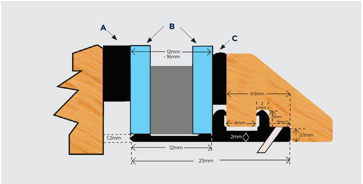
For Ventilated & Drained Bottom Timber Beads
