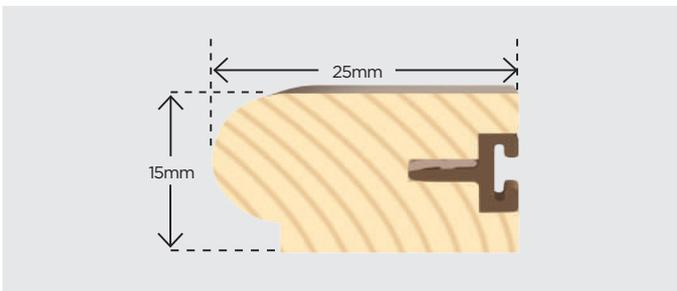
Timber Staff Bead 25mm x 15mm with Carrier & 6.5mm Pile & Fin
