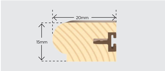
Timber Staff Bead 20mm x 15mm with Carrier & 6.5mm Pile & Fin
