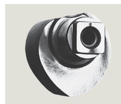
The heart-shaped cam and the linear drive mechanism which characterise all dormakaba cam-action door closers produce a rapidly decreasing opening torque, so greatly reducing the amount of effort required.
