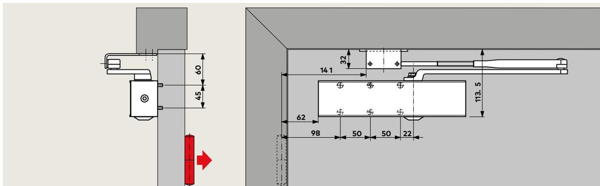
With parallel arm application, the backcheck comes in later at between 85° and 90°, depending on the door thickness and projection of
