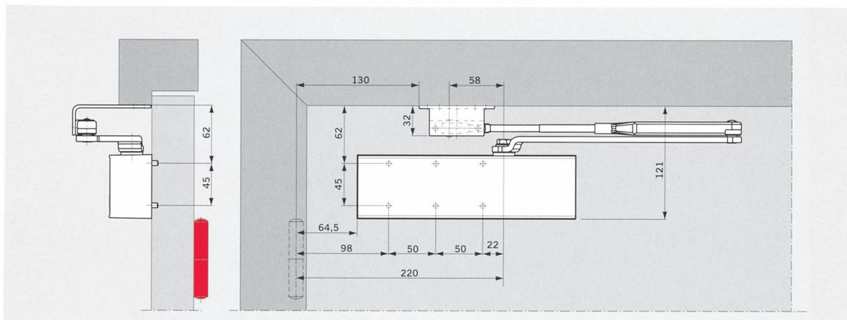
With this fixing method, the max closing force is approx. 20 Nm (for doors up to 950mm) Parallel-arm bracket (accessory) necessary
