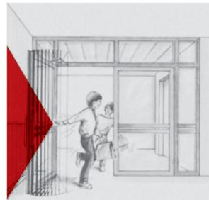
If the dormakaba TS 72 is installed with a hold-open arm, the doors can be held open at any desired point (up to approx. 150°).
