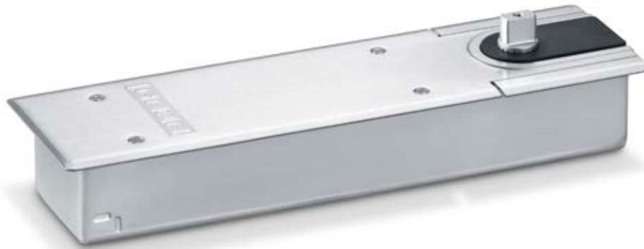
Floor spring for single leaf single and double-action doors of up to 1400 mm leaf width with adjustable closing force EN 3-6 and with hold-open function that can be switched on and off
