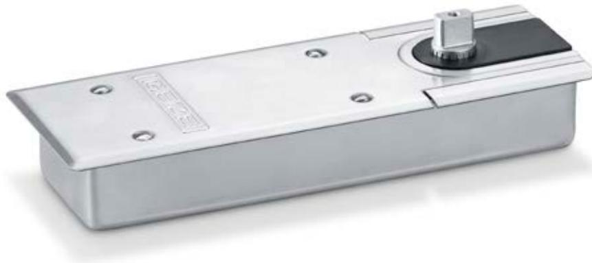
Floor spring for single leaf single and double-action doors of up to 1100 mm leaf width with adjustable closing force EN 1-4 and with optional hold-open function
